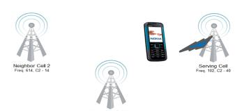
The handset is camped on channel 102 as it has the highest C2 value. The phone switches to a neighbor-cell when its C2 is higher than the Serving-cell.
