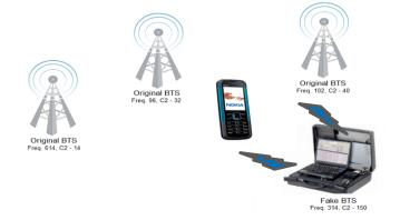
An active GSM interceptor is running its BTS, transmitting a C2 value of 150 and forcing the phone to camp on it. The phone will switch to fake-BTS with the highest C2.
